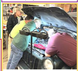
Many thanks to the Wednesday Night gang for working on Fr. Joe's old Jeep that developed an oil leak. With 151,000 miles, the seals are getting old and brittle, so new head gaskets had to be installed. Hopefully it will give Fr. Joe a few thousand more miles of reliable around town driving.
